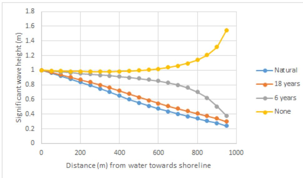
Fig. 1. Dissipation seen through wave height decrease as wave travels towards the shoreline for drag coefficient  $C_D = 1$ .
